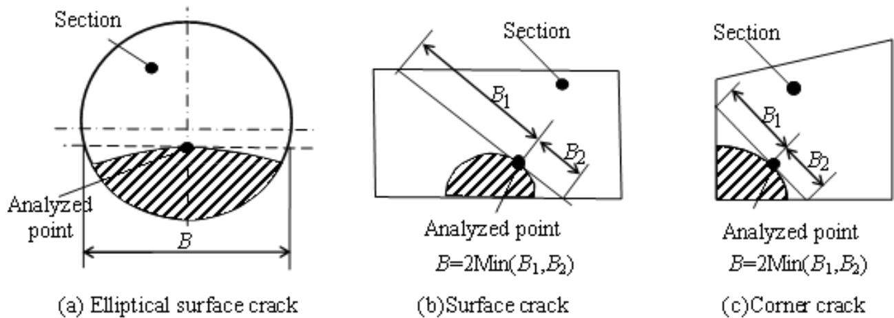
Fig. (1). Fatigue crack and the definition of equivalent thickness  $B$ .
