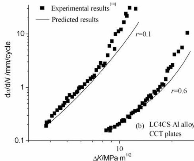
Fig. (6). The  $da/dN$ - $\Delta K$  curves of LY12CZ and LC4CS aluminum plates.
