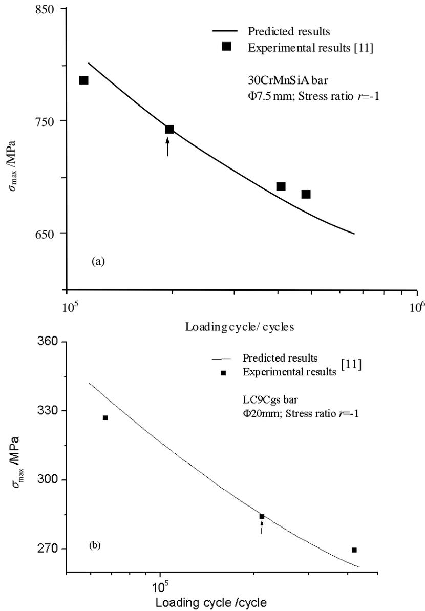
Fig.(2). The S-N curves of the rotating-bending round-bars.
