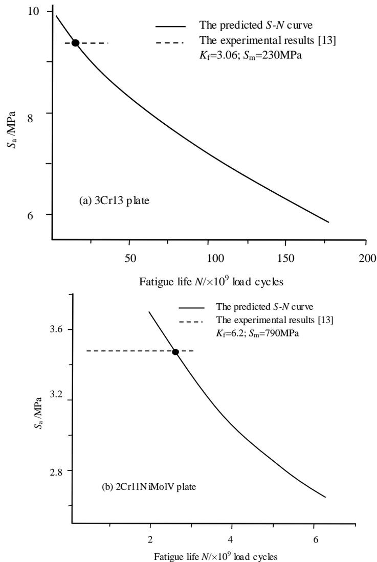
Fig. (4). The  $S$ - $N$  curves for 3Cr13 and 2Cr11NiMoIV plates.
