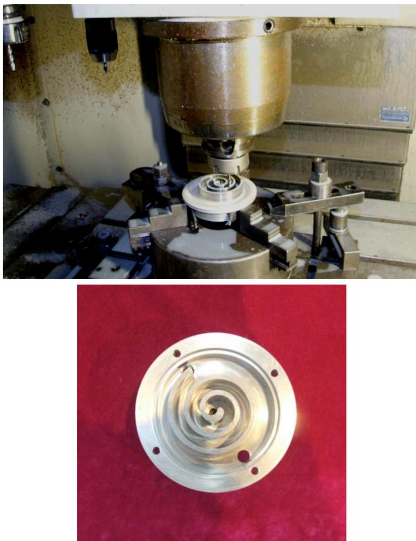
**Fig. (9).** Manufacturing process and the scroll model.
