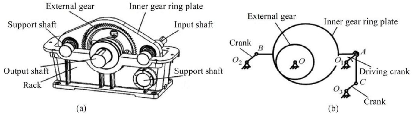
Fig. (1). Structure of one kind planetary gear reducer with a single ring plate and three cranks.
