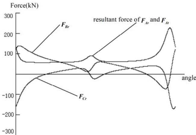
Fig. (5). Stress calculation results graph of the inner gear ring plate.
