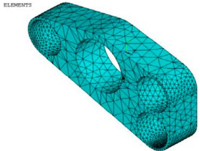
Fig. (6). Meshing situation of the inner gear ring plate.
