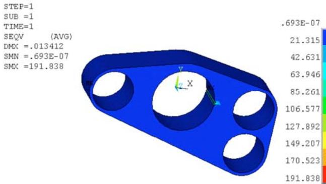
Fig. (8). Equivalent stress diagram of the inner gear ring plate.
