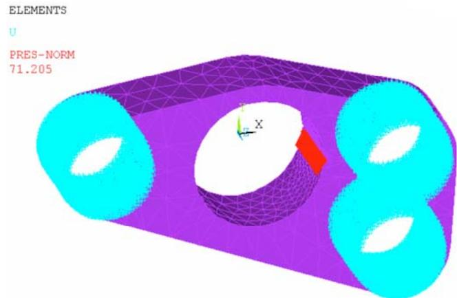
Fig. (7). Finite element model of the inner gear ring plate.
