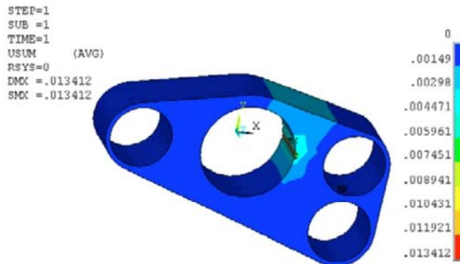
Fig. (9). Composite deformation diagram of the inner gear ring plate.
