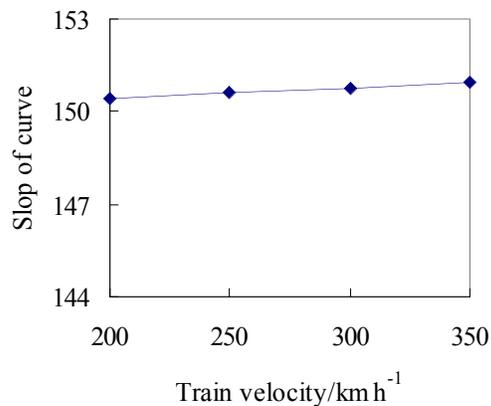
**Fig. (4).** Curve slope *versus* speed.
