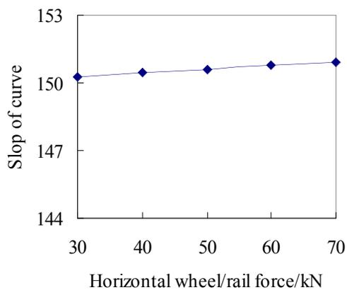
**Fig. (5).** Curve slope *versus* horizontal wheel/rail force.
