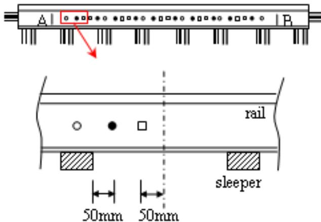
Fig. (3a). Sketch of sensor locations in simulation calculation.
