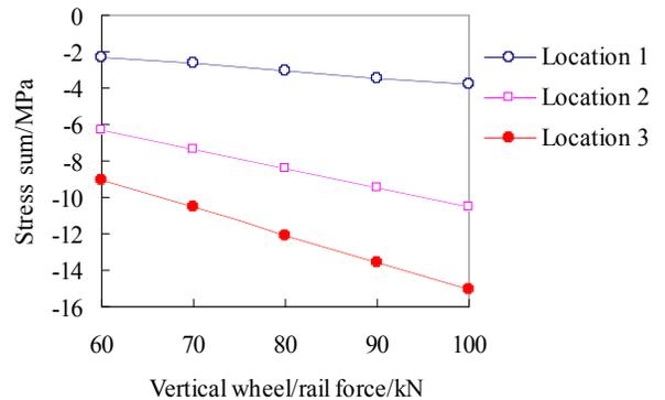
Fig. (3b). Relationship of stress versus vertical wheel/rail force.
